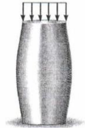
Compression causes material to bulge out
