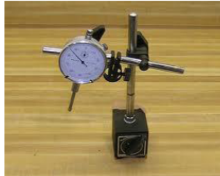
Dial Strain Gauge is used to measure the mid span deflection \delta
